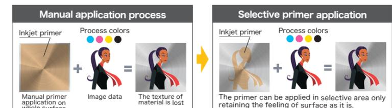
As the primer, PR-200 is applied simultaneously with color printing, the PR-200 applying only to the necessary part of material is possible, too. Therefore the texture of the base material that was lost by conventional manual primer applying can be maintained.
