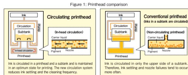
Figure 1: Printhead comparison
