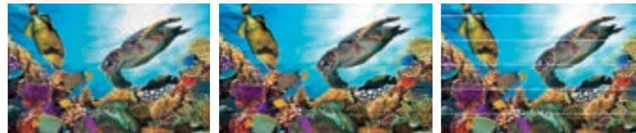
Improper dot position Overlap/Black streaks (Insufficient feeding amount) Gap/White streaks (Excessive feeding amount)
